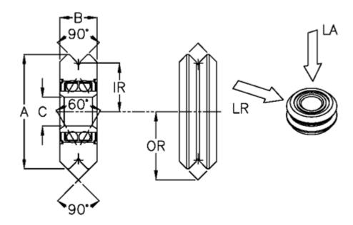
$\begin{array}{ll} \mbox{Diameter A} & = 45.80 \\ \mbox{Hole size C} & = 12.00 \\ \mbox{Internal radius IR} & = 19.05 \\ \mbox{Outer radius OR} & = 27.00 \\ \mbox{Width B} & = 15.88 \end{array}$
